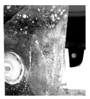
This is erosion corrosion on a rudder blade caused
